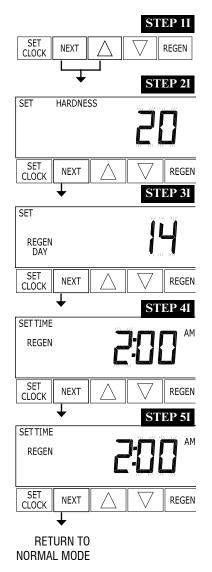
**STEP 1I** - Press NEXT and ▲ simultaneously for 3 seconds.
