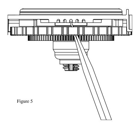
The drive cap assembly contains the drive cap, the main drive gear, drive cap spline, piston rod and various other parts that should not be dissembled in the field. The only replaceable part on the drive cap assembly is the o-ring. Attached to the drive cap assembly is the main piston (down flow or up flow) and if a regenerant is used, a regenerant piston.
